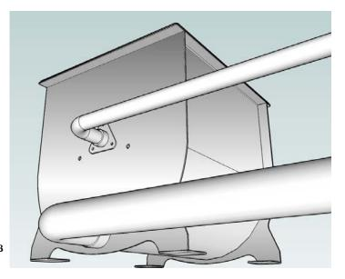
The meter case, metering drum, bearing brackets, bearing wheels, and inlet spout shall be made of stainless steel. A rotating, cylindrical drum of six scroll-shaped chambers measures the liquid by volume. Each compartment shall have two interior baffles attached to the side walls/heads of the drum to form a watertight seal where the baffle and wall meet.
