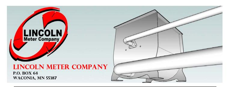
The meter case, metering drum, bearing brackets, bearing wheels, and inlet spout shall be made of stainless steel. A rotating, cylindrical drum of six scroll-shaped chambers measures the liquid by volume. Each compartment shall have two interior baffles attached to the side walls/heads of the drum to form a watertight seal where the baffle and wall meet.
